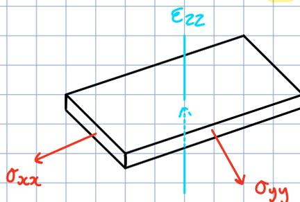
Stresses in y & z direction result in out of plane z strains due to Poisson
